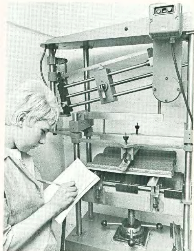
Transverse strength testing of a roofing tile.
