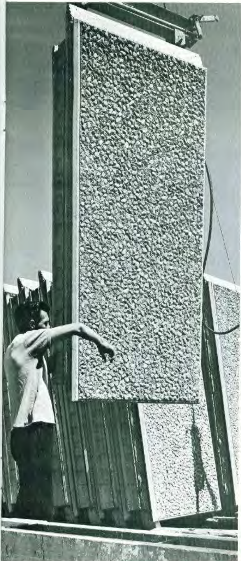
Left: Insulated gable cladding panels precast for a multi-storey project.
