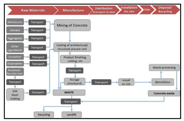
Different "unit processes" associated with the Cradle-to-Grave service life of architectural/ structural precast units.
