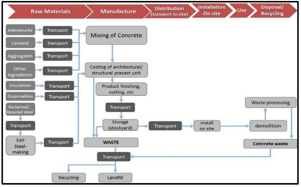
Different "unit processes" associated with the Cradle-to-Grave service life of architectural/ structural precast units.
