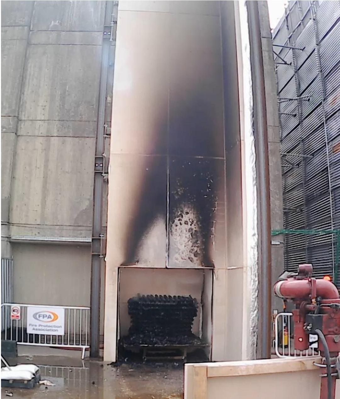
Figure 34 – Full façade post test
