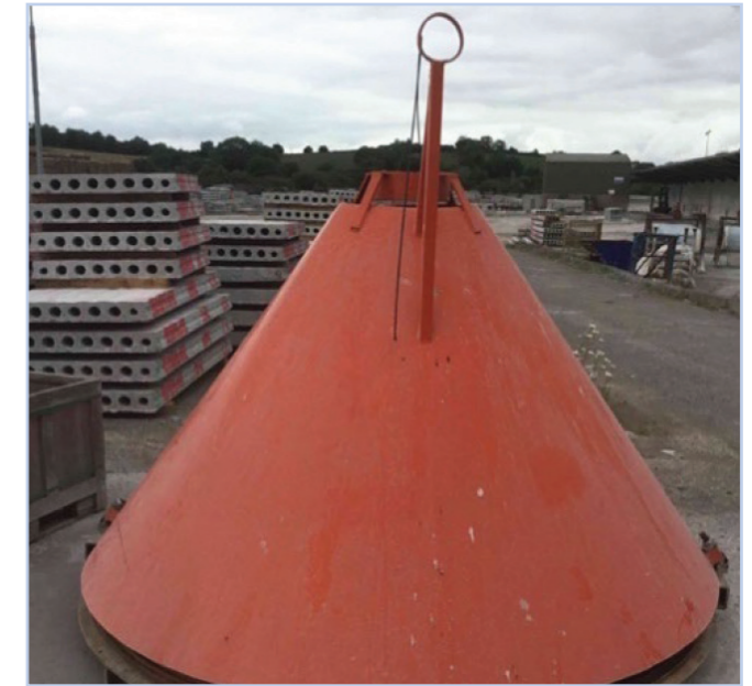
Figure 4.12 Cover lifted by forklift truck protecting wire from the elements.
