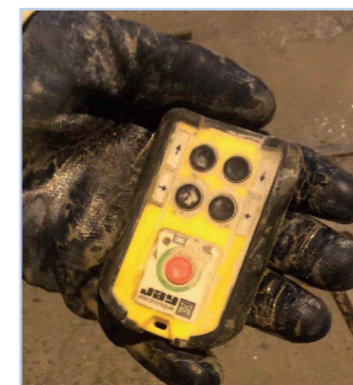
Figure 7.4 Multi-stressing remote control, allowing a greater distance from stressing operations.
