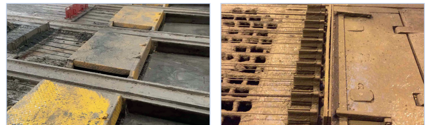
Figure 7.16 Left: Enclosed dead-end hollowcore. Right: Button head end guard.
