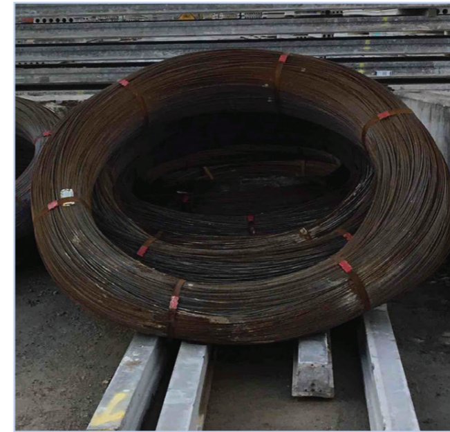
Figure 4.11 Poor storage - Risk of wire damage from concrete batons and the elements.
