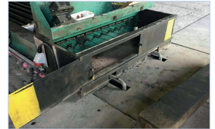
Figure 7.21 Sliding cover used to enclose stressed wires.
