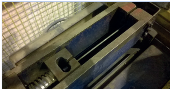
Figure 6.15 Button head destruction test.
