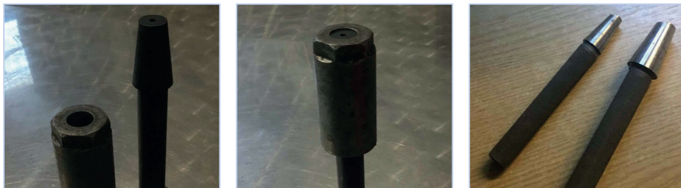
Figure 6.3 Steel barrel insert tools for measuring barrel wear.
