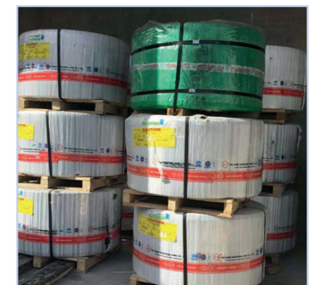
Figure 4.7 Strand coil laid ‘eye to the sky’.
