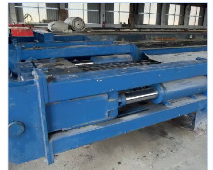
Figure 7.3 Multi-stressing mould in tensioned position.
