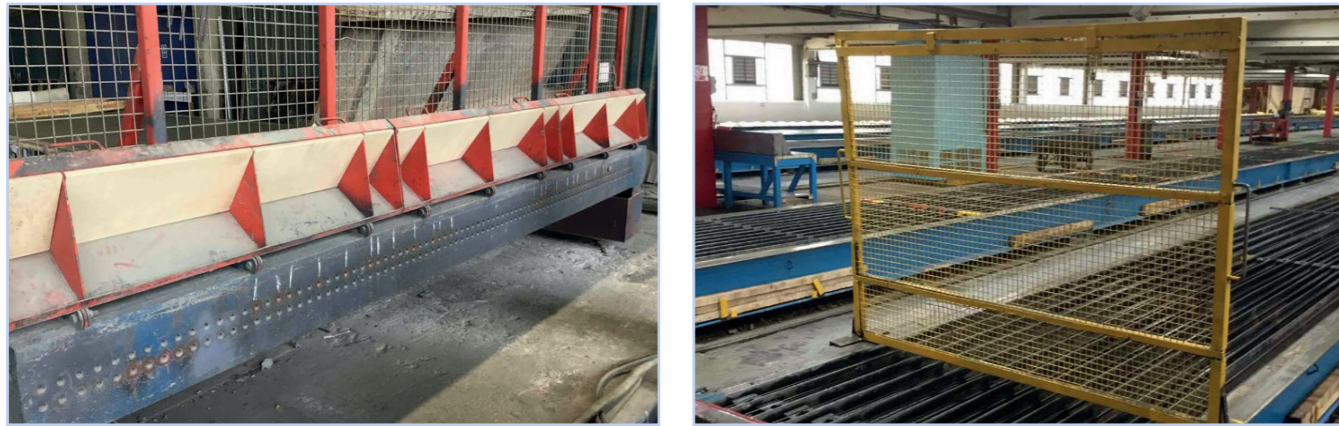
Figure 7.17 Left: Drop down live end guard with wooden insert. Right: Upright stressor guard.
