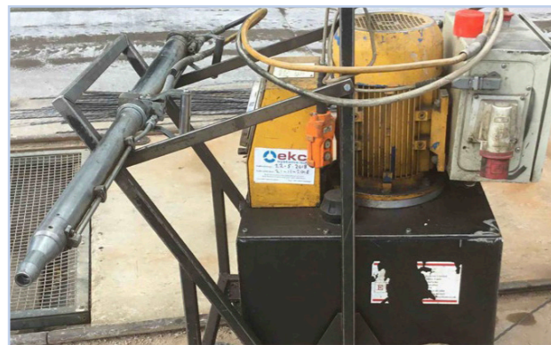
Figure 3.1 Single wire/strand stressing with a jack.
