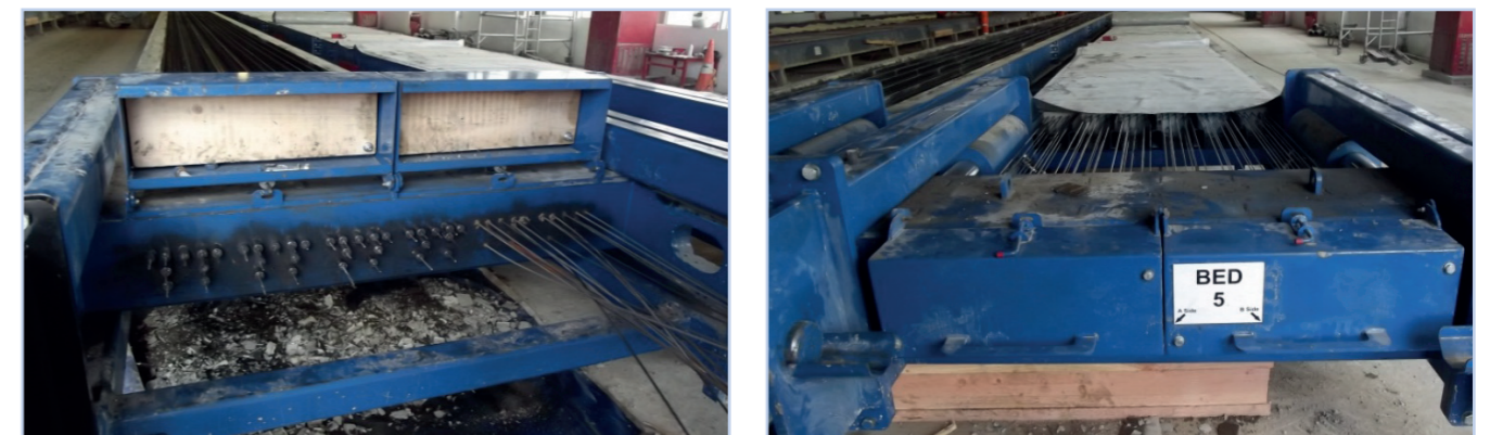
Figure 7.15 Stressing end of a wet-cast T-beam. Left: Guard raised showing timber insert used to absorb impact. Right: Guard lowered to contain all prestressed wires/strands.
