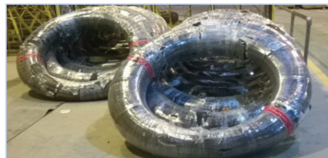
Figure 4.10 Wire storage in protected area, under cover and no standing water, etc..
