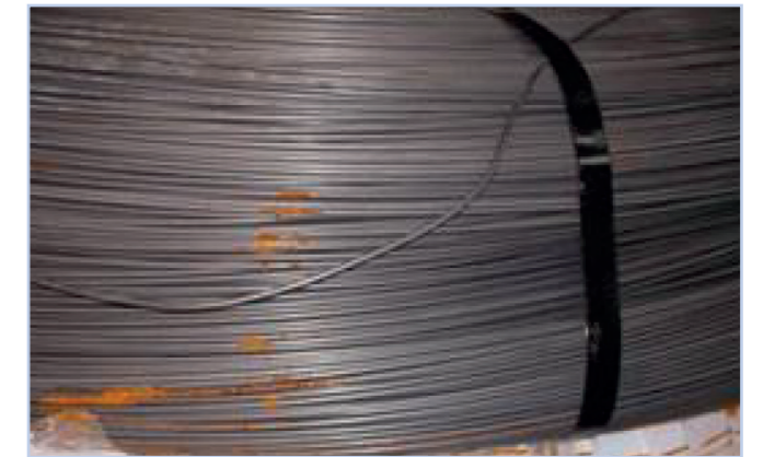
Figure 4.20 Wire kinked while still coiled.
