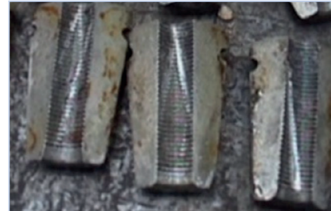
Figure 6.4 Wedges with evidence of slippage.
