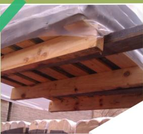
The loaded pallet should be sufficiently secured to the trailer bed to withstand any forward or sideways force. This is the responsibility of all parties, not just the driver.
