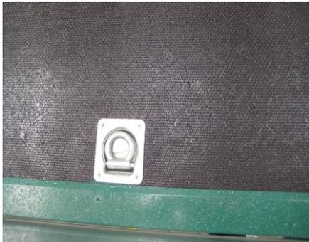
**Fig 1.** Care must be taken when using this type of floor mounted lashing point like the above as they are usually only rated to 500 daN (kg).
