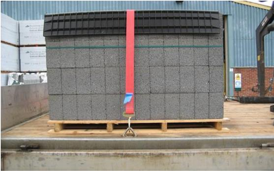
**Fig 6.** Corner protectors are very good at spreading the strapping forces over much greater area on packs of stacked items. Un-shrink-wrapped packs of blocks or bricks can be bound with the cling film type shrink wrap to prevent the loss of single items.
