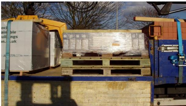
**Fig 4.** To increase the effectiveness of the lashing on low height products, or if due to width limitations requiring having to lash over drop side doors, packing of the product to increase height can be very effective as in the picture.
