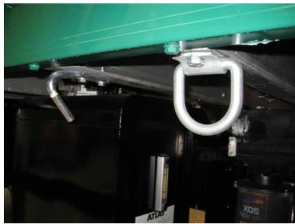
**Fig 2.** The two-bolt mounting lashing point above is available at a rating of 2,500 daN (kg) when the correct mounting bolts are used. These can be retro-fitted in place of rope hooks.
