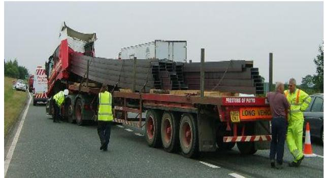
**NB: if more than 50% of the height of the load stands above the headboard, additional forward load restraint must be used to compensate for the lack of blocking**
