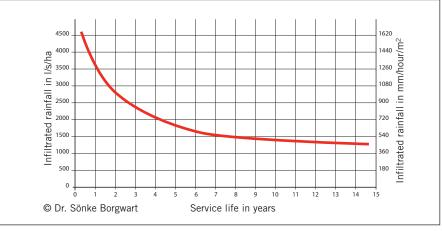
Typical reduction of surface infiltration rate over time.
